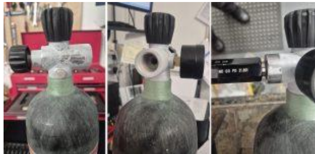
Unmarked valve thread failure
