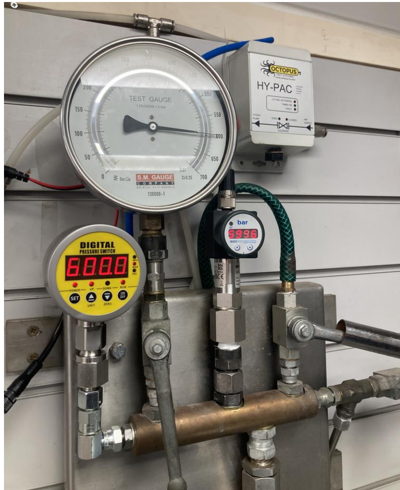
Image 2: Testing to 600 bar
