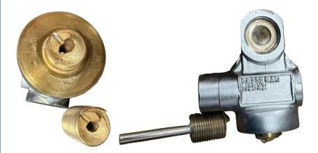
Modification of valves and threads in this way, without manufacturer authorisation and safety recertification of the valve, is potentially very risky. The centre acted correctly by informing the owner who agreed to the replacement of the valves with proper M18 alternatives.
