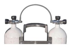
The challenge was that the CE EN144-1 M25x2 LOLA valves are marked as rated to 200 bar, and the 7-liter Eurocylinder Systems AG (ECS) cylinders are marked as working pressure 230 bar.
