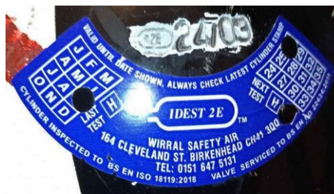
Next test incorrectly punched out
