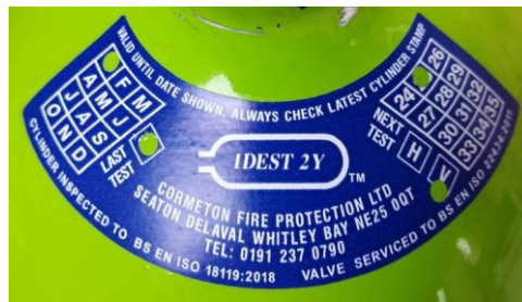
Last test incorrectly punched out
