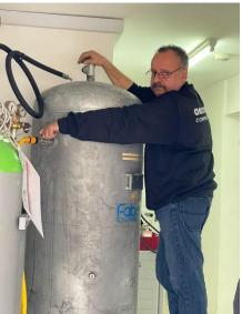
With the vessel prepared, normal procedure was followed for the test. Using a manual pump, the pressure was increased to test pressure and held for 20 minutes.
