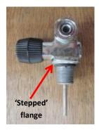
If a test centre comes across such a combination during a test, the 'O' ring must be removed and replaced **WITH THE BESPOKE WASHER** that these valves are designed to have. The top of the cylinder neck should be checked carefully for any consequent damage. If no resulting damage is found, then the cylinder can be hydraulically tested.
