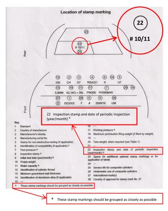
Providing the cylinder passes the test applied, whether it is a Volumetric or Proof test, then the stamp must be punched into the shoulder of the cylinder. Paint should be removed using a scraper and then the stamp is punched into the metal of the shoulder using metal punches and a lump hammer to apply the force. A thin coat of paint should be applied to protect the cylinder but not so thick as to obscure the stamp details.
